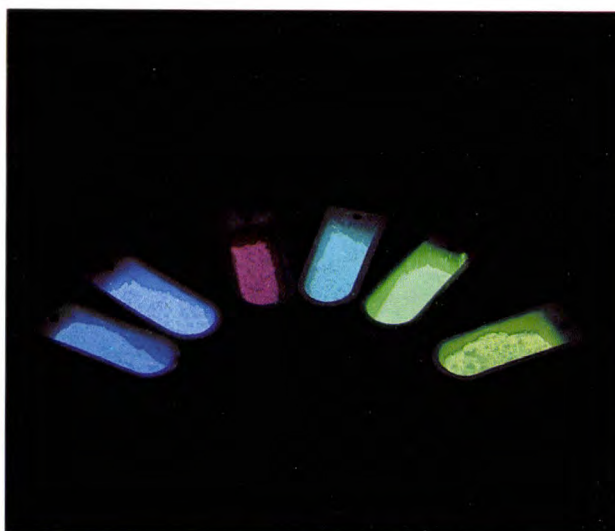
Fig. 1. Some of the phosphors dealt with in this article, irradiated by an ultraviolet lamp. From left to right: two blue phosphors, \text{Sr}_{0.9}\text{La}_{0.1}\text{Mg}_{0.1}\text{Al}_{11.9}\text{O}_{19}:\text{Eu}^{2+} (i.e. Sr-La-Mg aluminate activated with divalent europium) and \text{BaMgAl}_{10}\text{O}_{17}:\text{Eu}^{2+} , the red phosphor: \text{La}_{0.68}\text{Eu}_{0.21}\text{Mn}_{0.60}\text{Al}_{11.52}\text{O}_{19.11} , the blue-green phosphor: (\text{Ca},\text{La})\text{Al}_{12}\text{O}_{19}:\text{Eu}^{2+},\text{Mn}^{2+} and the two green phosphors: \text{BaMgAl}_{10}\text{O}_{17}:\text{Eu}^{2+},\text{Mn}^{2+} and \text{Ce}_{0.67}\text{Tb}_{0.33}\text{MgAl}_{11}\text{O}_{19} .
