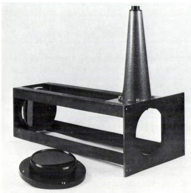
Fig. 5. External optical systems for the LEP thermograph for microthermography ( above ) and macrothermography ( below ).
