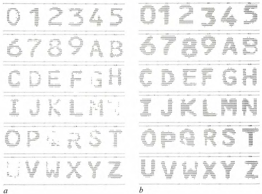
Fig. 8. The output pictures obtained with a set of machine-print characters of good quality (a), poor quality of low-contrast type (b), poor quality of 'heavy' type (c), all processed by an OCR machine that included a camera with a double threshold. The material for figs. 8b and 8c was also processed by an X-1300 machine (fig. 9).
