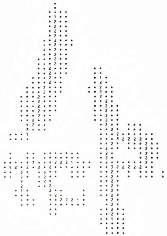
Fig. 12. An example of severely mutilated handprint output. The original, the number 4 written with a blunt pencil under heavy pressure, had limbs so wide that the defocused array (fig. 4) could not see the background in some locations. Increasing the field of view of the defocused array could overcome this difficulty, but the sensitivity of the camera would then decrease.
