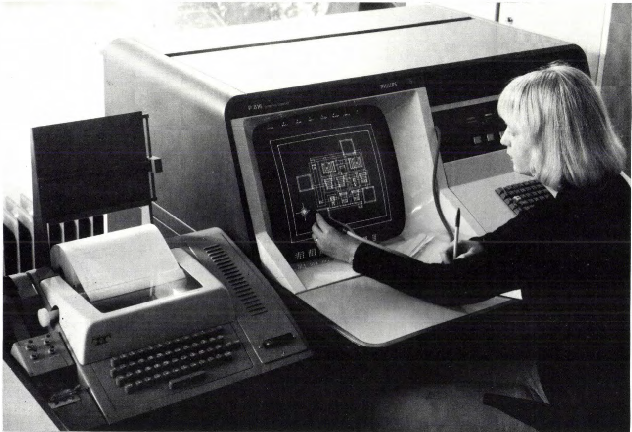
Fig. 16. Design and correction of a layout with a graphical display. The light pen is used for indicating and moving figures on the screen; the keyboard ( right ) is used for typing in new values.
