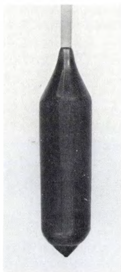
Fig. 4. A pulled BSO crystal with a diameter of 42 mm; its weight is 1.4 kg.
