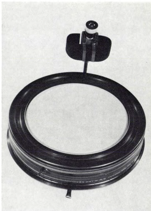
Fig. 6. An X-ray image intensifier with metal conversion foil and electron-intensity amplification by means of a channel plate. The photograph shows the glass output window with the fluorescent layer. The getter-ion pump, which remains permanently connected, removes the residual gases released from the channel plate during operation. In this construction there is no room to incorporate a conventional absorption getter of sufficiently large capacity.
