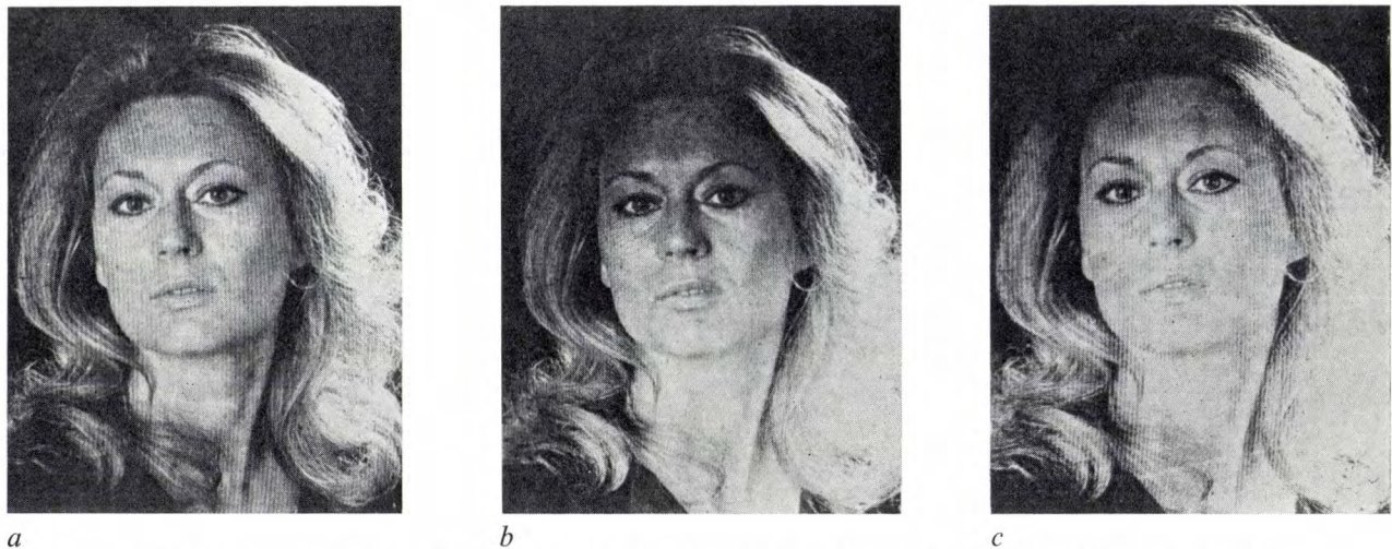
Fig. 7. Reconstruction of holograms during the various stages of thermal fixing. a ) Direct image of the object, seen through the crystal. b ) Reconstruction during recording at 150 °C. c ) Reconstruction after fixing.
