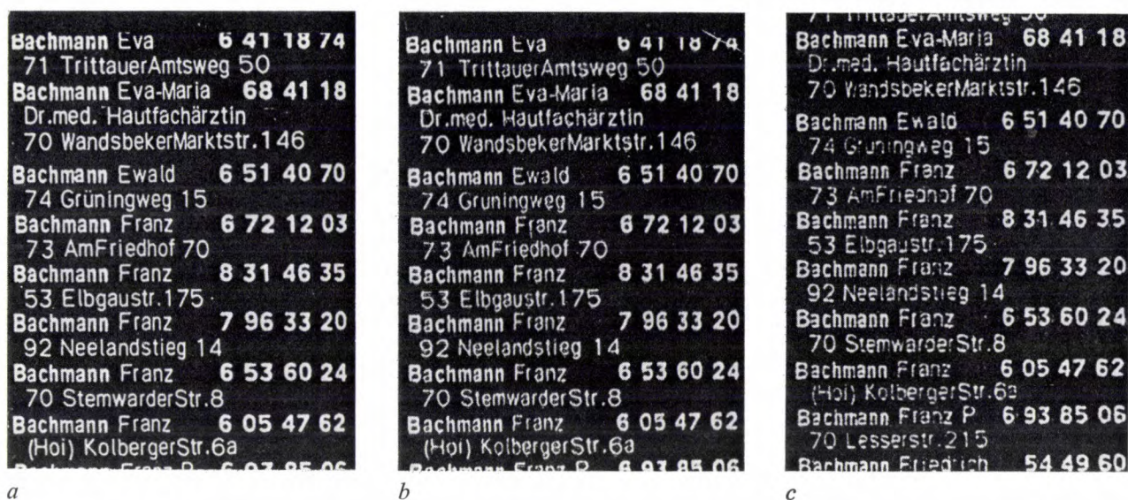
Fig. 10. Reconstruction of images with high information density. a ) Object. b ) Direct image seen through the crystal. c ) Reconstruction of a thermally fixed hologram, recorded at 150 °C. Area of crystal 50 mm 2 , thickness 5 mm.
